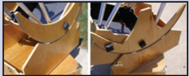
Figure 10. Altitude bearings. One of them can accept an extension spring mount as a virtual counterweight.
