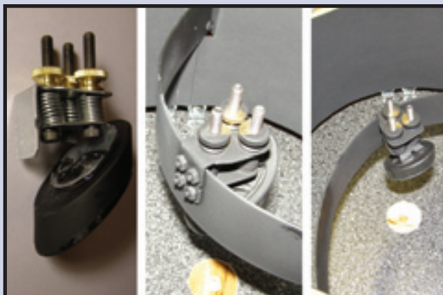
Figure 4. The low profile spider can fit into a short secondary cage.
