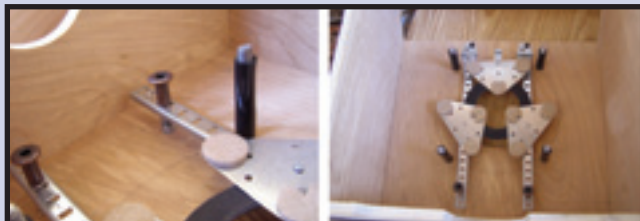
Figure 6. The mirror cell detail. The front protective screws were later moved to the sides, the sling was installed on them (not shown).
