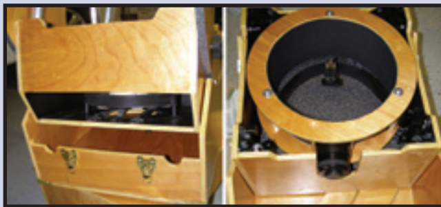
Figure 5. The front wall and the bottom of the mirror box are smaller in order to create an open notch. This allows to design a lower rocker box and let the air circulate and accelerate the primary mirror cooling. For storage, the mirror box must accommodate the secondary cage with the focuser.
