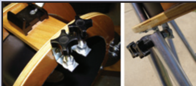
Figure 7. Attachment of the upper part of the truss tubes.
