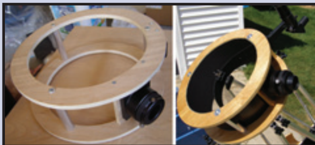
Figure 3. The secondary cage takes shape. Kydex was used for baffling.
