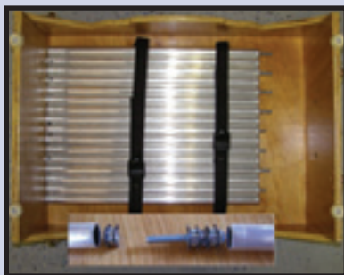
Figure 8. Attachment of the lower part of the truss tubes.
