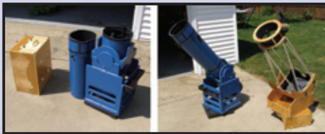
Figure 1. Splitting the Sonotube is not enough for a small car owner. The “chest design” saves the day!
