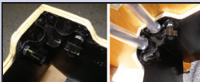
Figure 8. Attachment of the lower part of the truss tubes.
